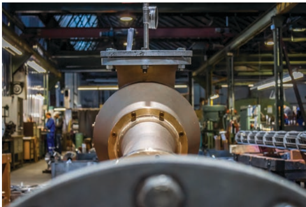
Jet ejector with suction power of more than 500 cubic metres per hour
