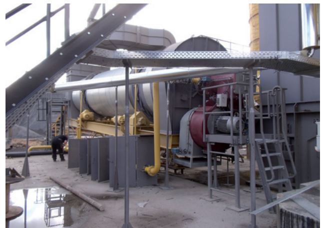
In operation for firing dusts, oils and gases at asphalt mixing plants.
