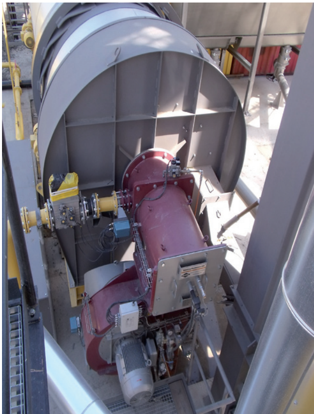
For Monoblock burners the combustion air blower is integrated at the burner.
