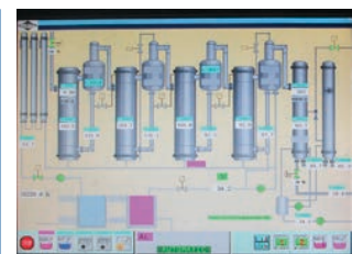
Control panel of a caustic recovery plant
