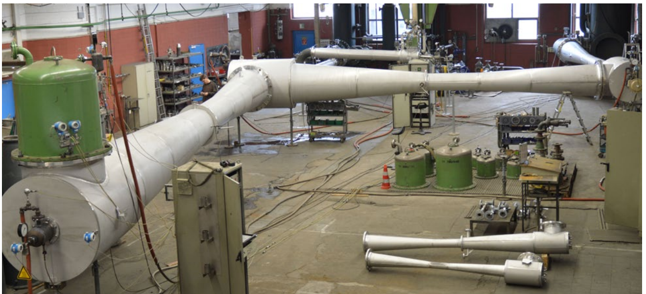
The three jet ejectors directly connected with one another create a low vacuum of 0.1 mbar on the test rig at Körting Hannover AG
