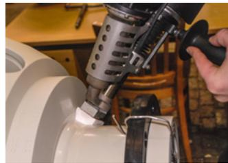
Welding a stub joint
