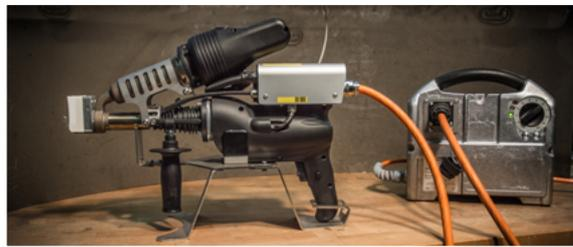
WE welding device MUNSCH MAK – 25 with „Powerbox“ high-frequency drive
