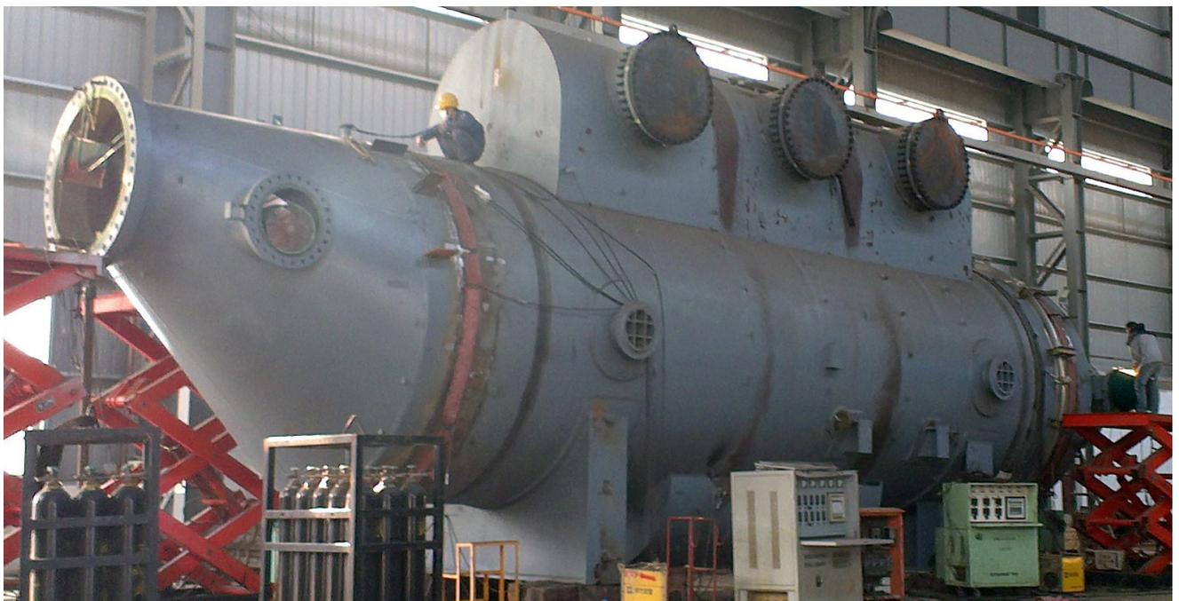
The bigger turbine condenser being manufactured in China. The vast dimensions indicate the magnitude of the project.
