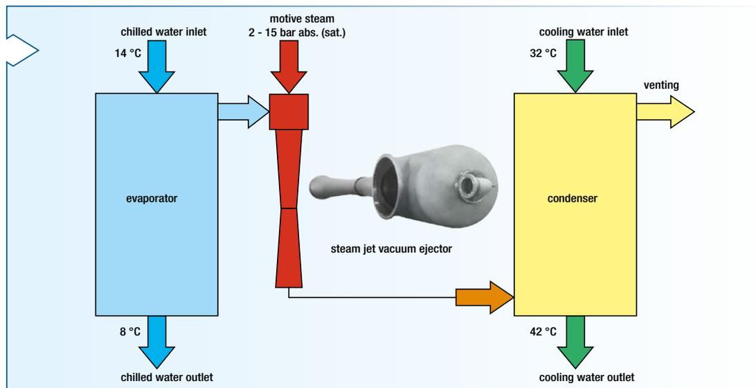
Schematic diagram: steam jet chilling plant
