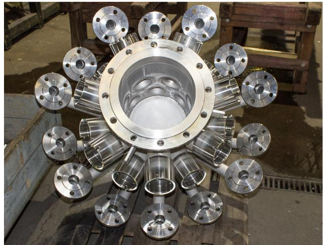
The 14-jet ejector during production
